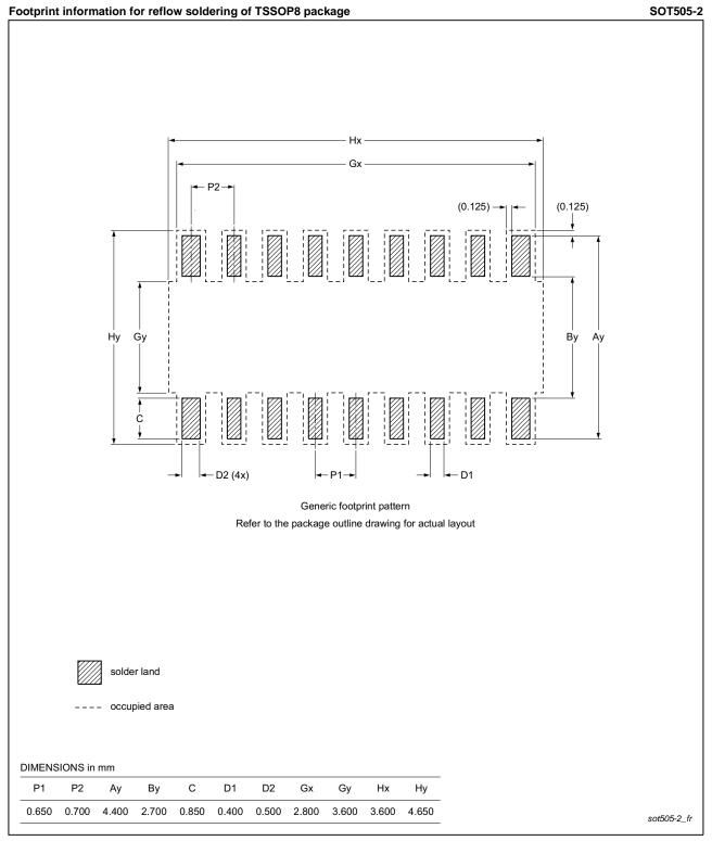
Fig 25. PCB footprint for SOT505-2 (TSSOP8); reflow soldering
