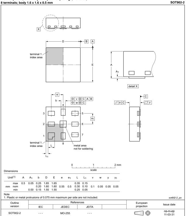
XQFN8: plastic, extremely thin quad flat package; no leads; 8 terminals; body 1.6 x 1.6 x 0.5 mm
