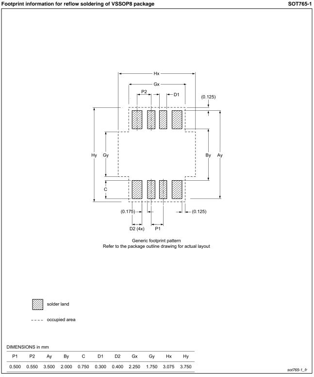
Fig 26. PCB footprint for SOT765-1 (VSSOP8); reflow soldering
