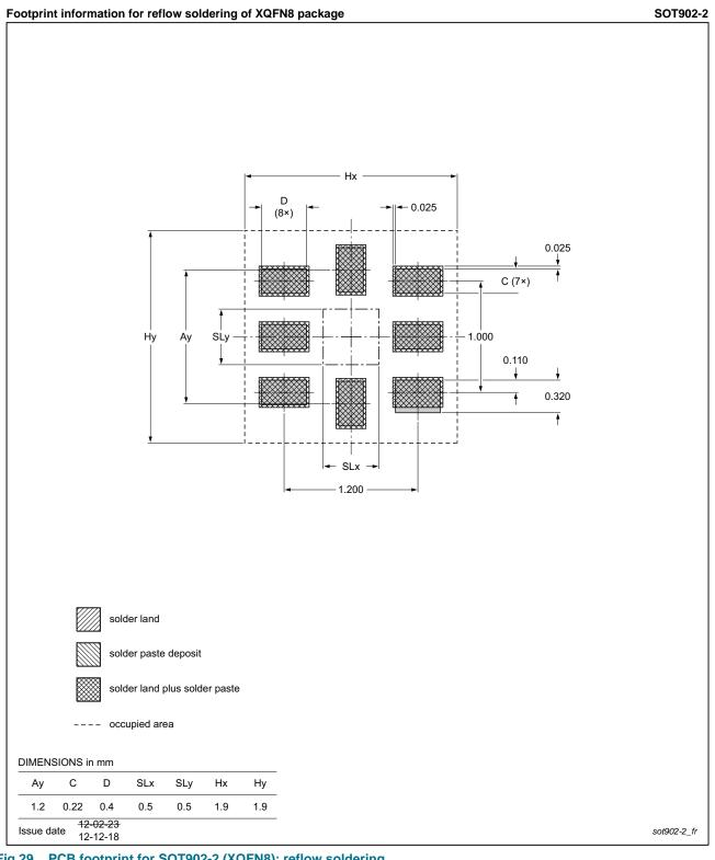
Fig 29. PCB footprint for SOT902-2 (XQFN8); reflow soldering
