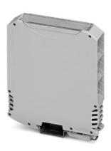
Electronic housing consisting of: Housing shells left and right, front plate, transparent cover, metal foot catch and spring, open housing, 24-pos. (6 x 4 pos.), width: 22,5 mm, color: Light gray
