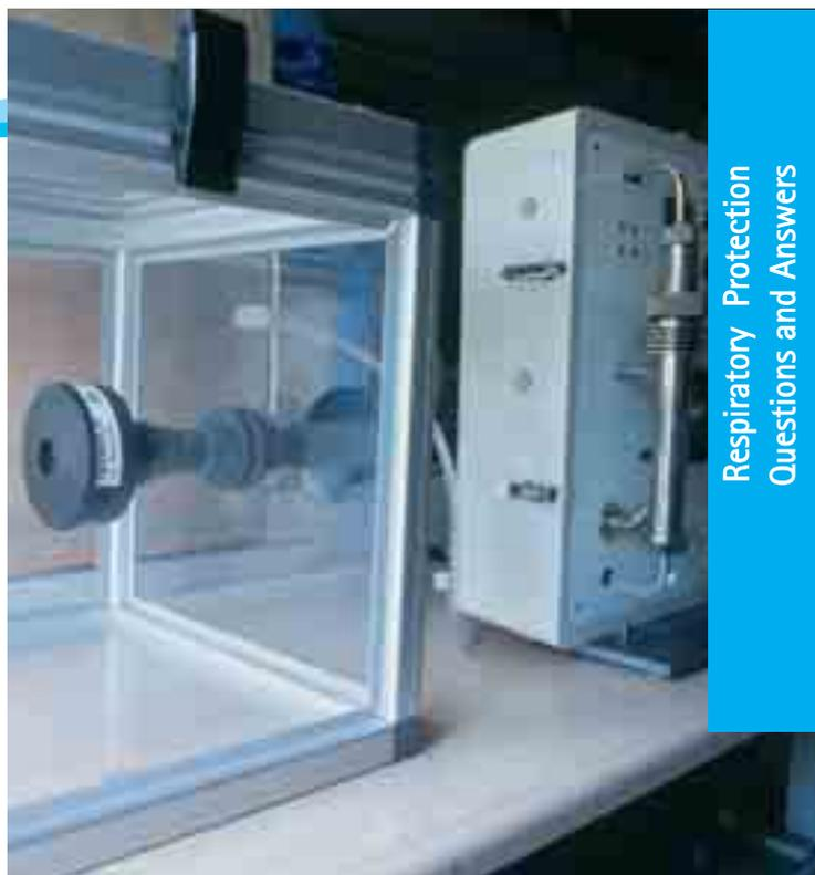
DIN Filter Penetration Testing
