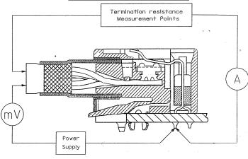
System resistance equals millivolt drop (mV) divided by test current (A) (Conductor resistance will be deducted from measurement).
