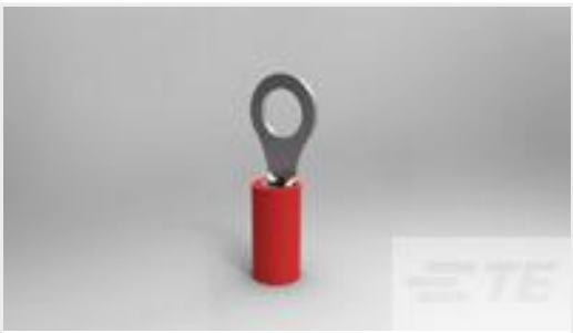
TE Part #171508-2 PIDG WIRE TERM, #8, 22-16 AWG
