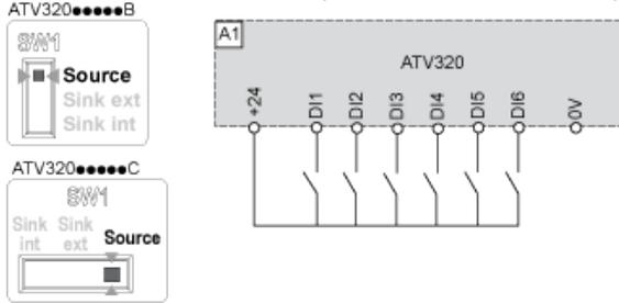
Switch SW1 set to "Source" position and use of an external power supply for the DIs.
