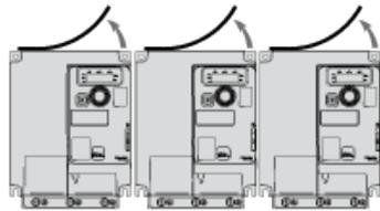
Mounting Type C: Individual, Ventilation Cover Removed
