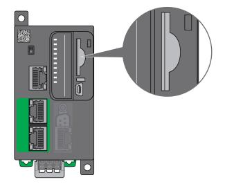
It is possible to set the Write-Control Tab to prevent write operations to the SD card. Push the tab up, as shown in the example on the right-hand side, to release the lock and enable writing to the SD card. Before using an SD card, read the manufacturer's instructions.
