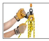
Release of the cam and passage of the rope through the brake integrated into the main moving side plate, allows comfortable and precise control when lowering.
