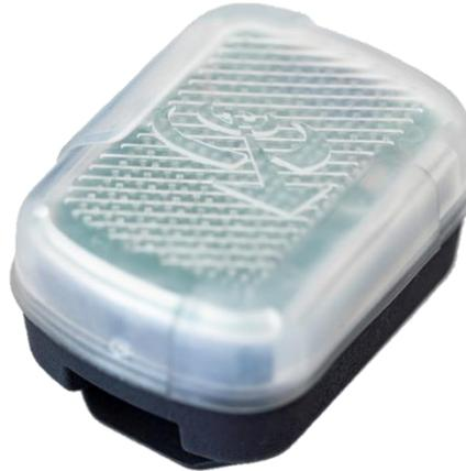
The TAG is a wearable device that allows the measurement of interpersonal distance by warning of the danger of excessive proximity between several people..
