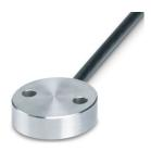
Lambrecht Meteo GmbH PV module temperature sensor consisting of Pt 100 Modbus converter and Pt 100 temperature sensor. The measurement value is provided via Modbus/RTU (RS-485).
