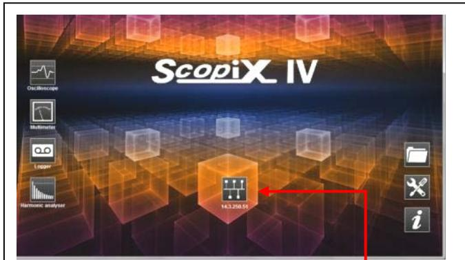
When you have obtained the IP address of the **Scopix** (DHCP or manual) using a browser, type 14.3.250.51/scopenet.html (for example) on your computer → this opens the screen shown opposite.
