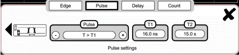
In all cases, the actual triggering is on the end-of-pulse edge:
