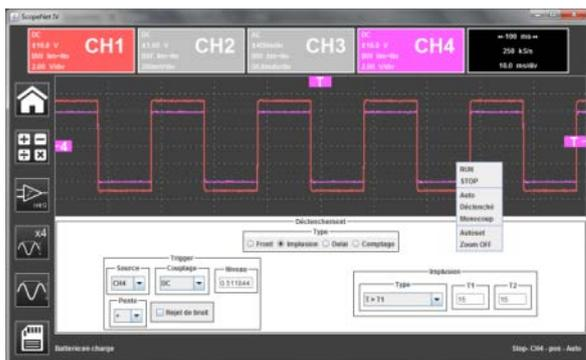
In "Oscilloscope" mode, **ScopeNet IV** proposes adjustments by a right click on the waveform: RUN/STOP, AUTO/TRIG/SINGLE/AUTOSET and ZOOM are easy-to-configure parameters.
