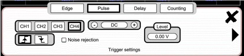
The edge is selected either in the "Trigger" tab or from the keypad and defines the limits of the analysis:
