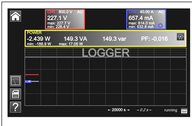
Each recording file contains 100,000 measurements per channel, at a rate of one measurement every 0.2 sec for 20,000 sec (approx. 5h30').
