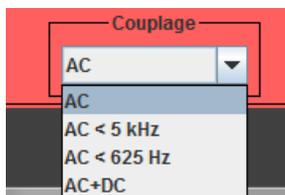
In MULTIMETER mode, the vertical configuration can be accessed by a click in the window shown opposite:
