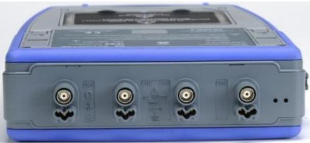
**ScopiX** uses **Probix intelligent probes and sensors**, which are recognized automatically when connected, giving the user active safety.
