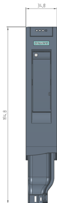
Figure A-4 Dimensional drawings of interface module IM 155-5 MF HF with strain relief
