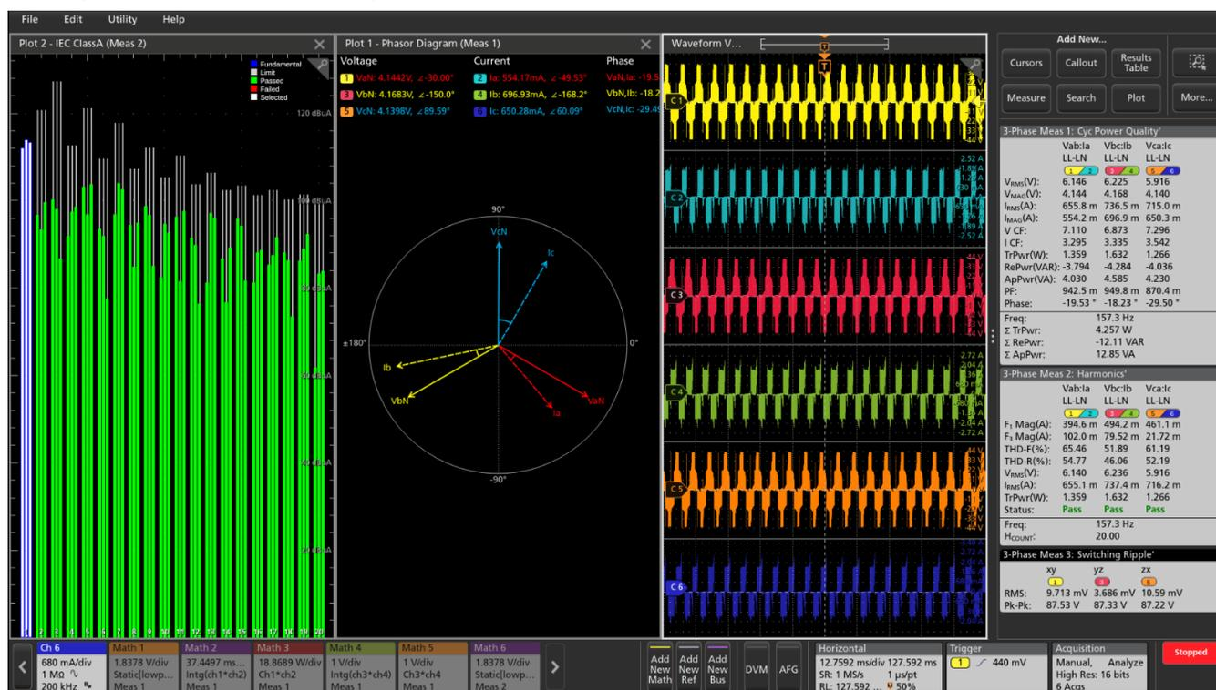
The power quality measurement provides an in-depth insight into the three-phase signals with an oscilloscope-based phasor diagram.
