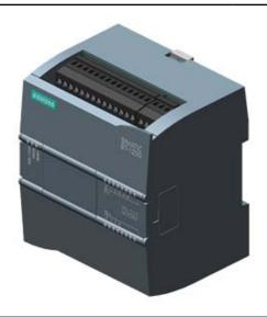
SIMATIC S7-1200, CPU 1211C, CPU COMPATTA, AC/DC/RELE', ONBOARD I/O: 6 DI 24V DC; 4 DO RELE' 2A; 2 AI 0 - 10V DC, ALIMENTAZIONE: AC 85 - 264 V AC CON 47 -63 HZ, 30 KB PER PROGR./SUPPORTO DATI
