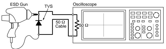
Figure 8. Diagram of ESD Clamping Voltage Test Setup
