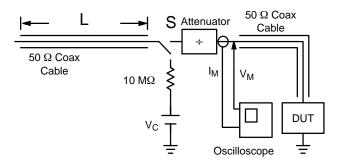
Figure 11. Simplified Schematic of a Typical TLP System
