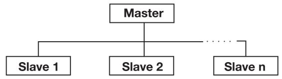
The master controls the data exchange, the slaves only have a response function. They are identified by their device address.
