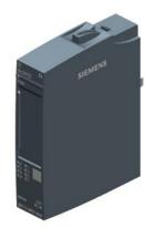
SIMATIC ET 200SP, Digital input module, DI 8x 24V DC Basic, type 2 (IEC 61131), sink input, (PNP, P-reading), Packing unit: 1 piece, fits to BU-type A0, Colour Code CC01, input delay time 0,05..20ms, module diagnostics for: supply voltage
