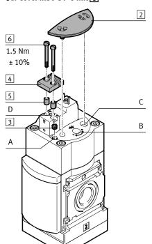
If the threaded pin 3 is not mounted at the factory:
