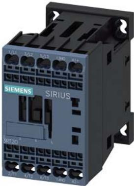
power contactor, AC-3e/AC-3, 12 A, 5.5 kW / 400 V, 3-pole, 24 V DC, 0.7-1.25\*  $U_c$ , with integrated suppressor diode, auxiliary contacts: 1 NO, spring-loaded terminal, frame size: S00, suitable for PLC outputs, no auxiliary switch can be added, upright mounting position
