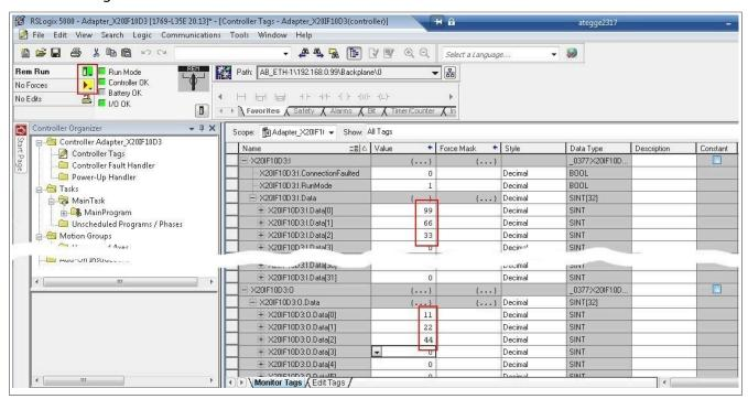
The online mode must be enabled as well. In order to force outputs, **Enable all I/O forces** must also be enabled.
