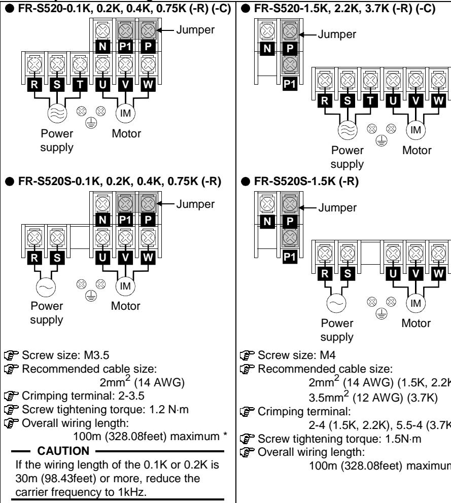
\* When automatic torque boost is selected in Pr. 98 "automatic torque boost selection (motor capacity)": 30m (98.43feet) maximum.
