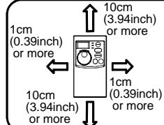
These clearances are also necessary for changing the cooling fan.
