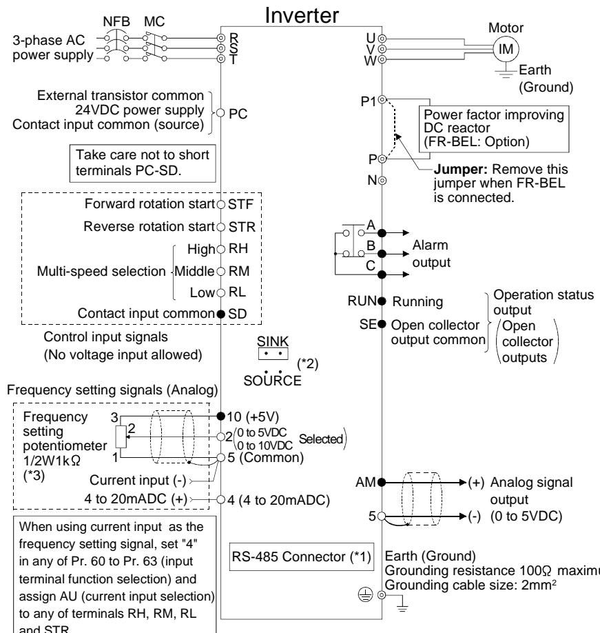
◎ Main circuit terminal, ○ Control circuit input terminal, ● Control circuit output terminal
