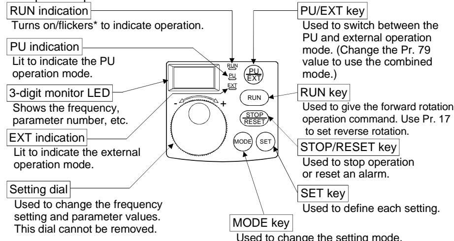
\*RUN indication On: Indicates that forward rotation operation is being performed.
