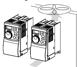
When containing two or more inverters, install them in parallel and provide cooling measures.
