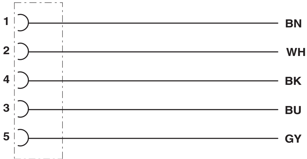
Contact assignment of the M12 socket
