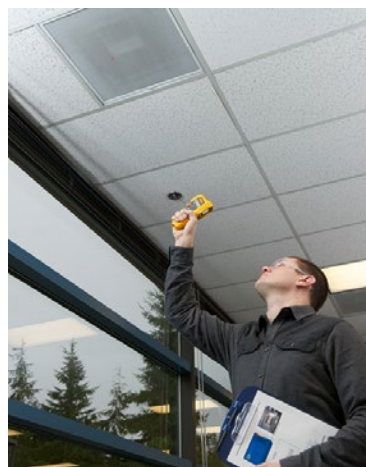
Checking the discharge temperature at air distribution ducts.
