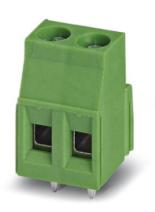
Printed circuit terminal block, nominal current: 16 A, rated voltage: 250 V, pitch: 5.0 mm, no. of positions: 3, mounting: Soldering, type of connection: Screw connection, connection direction from the conductor to the PCB:  $0^{\circ}$
