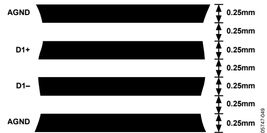
Figure 61. Arrangement of Signal Tracks
