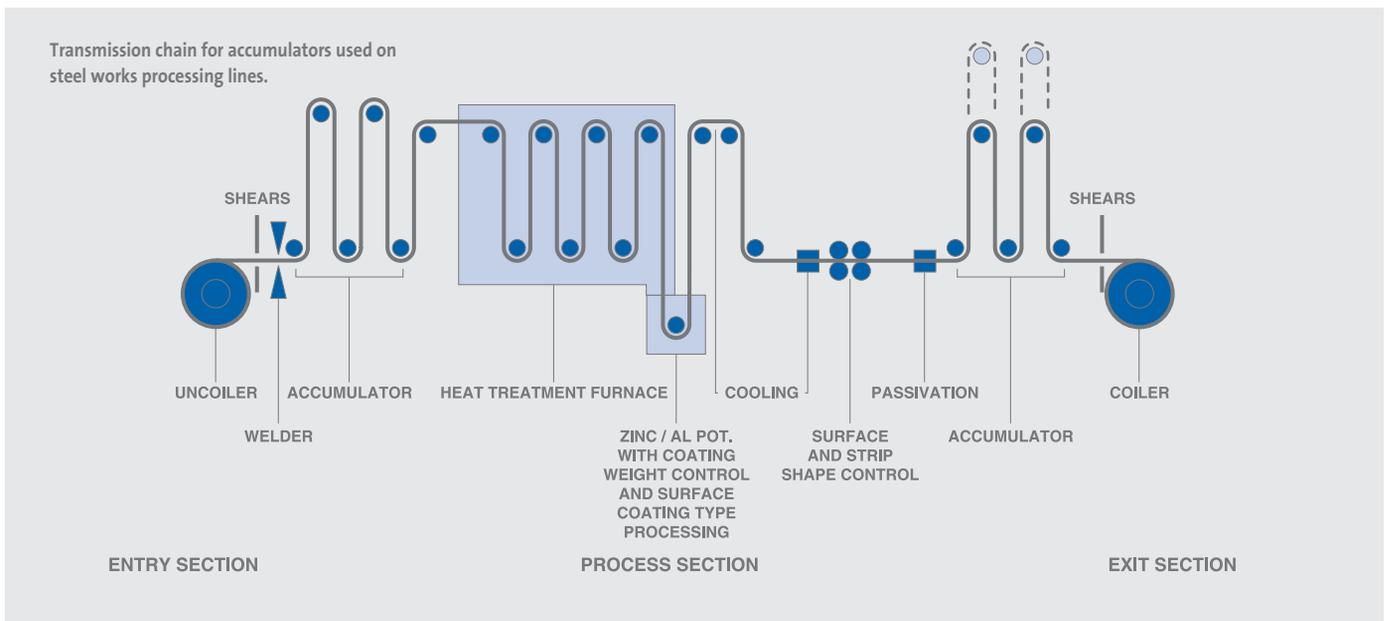
When coils of thin steel plate have been produced it is sometimes required to be coated - painted, galvanised or plastic coated.
