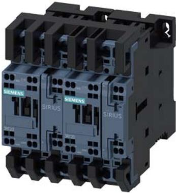
reversing contactor assembly, AC-3e/AC-3, 12 A, 5.5 kW / 400 V, 3-pole, 24 V DC, with integrated diode, spring-loaded terminal, electrical and mechanical interlock, auxiliary contacts: 2 x 1 NO
