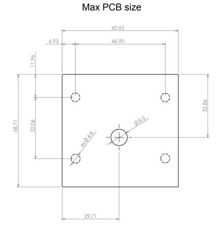
Dashed line shows outline of the mounting boss under PCB board Recommended mounting holes diameter ø3,5mm All dimensions are given within +/-0,5mm tolerance
