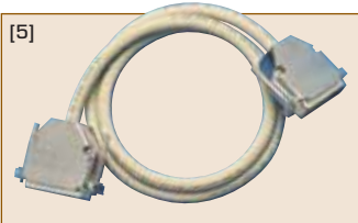
ME AK-D78/x: 0.25 m, 1 m, 2 m cable, 78-pin D-sub male - female (as HQ: 0.25 m, 1 m, 2 m length and 1 m open ends)
