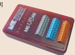
ME-UB Serie - ME-UBRE: 15-pin D-sub female, spring terminals. 8 relays type C. Expands TTL digital channels
