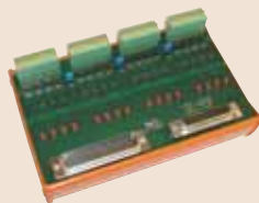
ME-63Xtend series - ME-632 EXT: 78-pin D-sub male, pluggable spring terminals. 16 opto-inputs. Expands TTL digital channels
