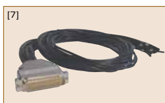
ME AK-D78/6000M-F/x: 0.25 m, 1 m, 2 m special cable, 78-pin D-sub male - female, for ME-6x00 (as M-OE/1: 1 m, open ends)
