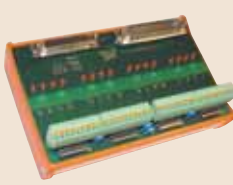
ME-63Xtend series - ME-633 EXT: 78-pin D-sub male, pluggable spring terminals. 16 opto-outputs. Expands TTL digital channels
