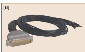
ME AK-D78/4000M-F/x: 0.25 m, 1 m, 2 m special cable, 78-pin D-sub male - female, for ME-46xx (as M-OE/1: 1 m, open ends)
