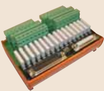
ME-63Xtend series - ME-631 EXT: 78-pin D-sub male, pluggable spring terminals. 16 relays type C. Expands TTL digital channels
