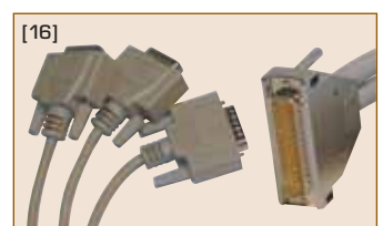
ME AK-D7815/1400: 0.5 m cable, 78-pin D-sub male - 25-pin D-sub male + 3x 15-pin D-sub male
