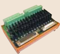
ME-63Xtend series - ME-635 EXT: 78-pin D-sub male, pluggable spring terminals. 16 solid state relays. Expands TTL digital channels
