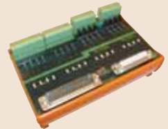
ME-63Xtend series - ME-634 EXT: 78-pin D-sub male, pluggable spring terminals. 8 opto-inputs/8 opto-outputs. Expands TTL digital channels
