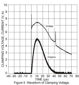
Current vs. Time (8/20µs, I/O to V<sub>SS</sub>)
