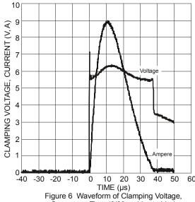
Current vs. Time (8/20µs, V<sub>CC</sub> to V<sub>SS</sub>)
