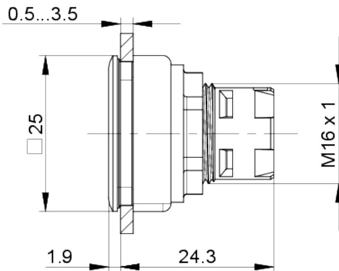
**Mounting hole drawing**
