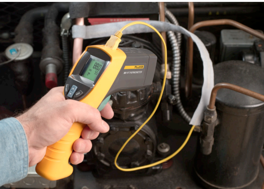
Measuring compressor line temperature with the Velcro K-type thermocouple for the Fluke 561 IR Thermometer.
