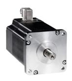
3-phase stepper motor - 13.5Nm - shaft Ø19mm - L=180mm - w/o brake - connector
