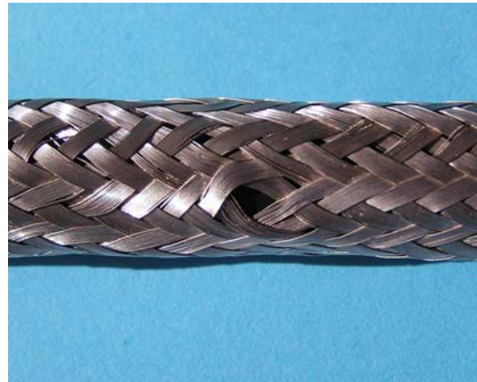
NOT ACCEPTABLE Window in Shield
