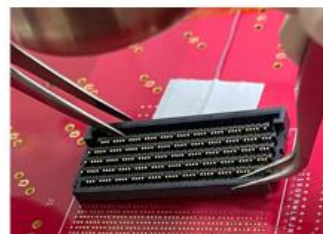
Step 8: Remove connector using tweezers
