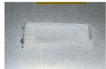
Step 4: Apply solder paste using mini-stencil
