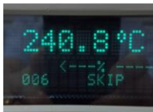
Step 7: Allow temperature on thermocouple to reach approx. 240°C
