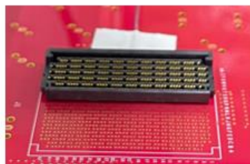
Step 8: Replace new connector
