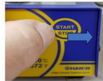
Step 3: Press Start / Stop on pre-heater
