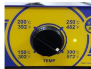
Step 4: Adjust temperature knob to 300°C
