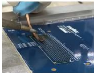
Step 2: Remove solder residue using solder-iron and wick
