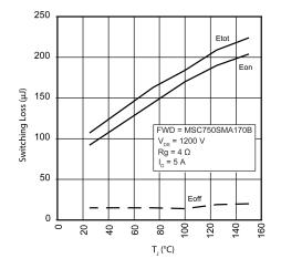
Figure 14 • Switching Energy vs. Temperature
