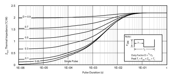
Figure 17 • Maximum Transient Thermal Impedance
