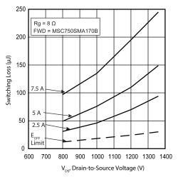
Figure 12 • Switching Energy vs. V<sub>DS</sub> & I<sub>D</sub>
