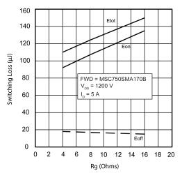
Figure 13 • Switching Energy vs. Rg
