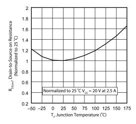
Figure 5 • RDS(on) vs. Junction Temperature
