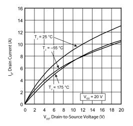
Figure 1 • Drain Current vs. V<sub>DS</sub>
