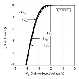
Figure 10 •  $I_D$  vs.  $V_{DS}$  3<sup>rd</sup> Quadrant Conduction
