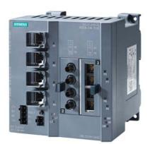
SCALANCE X308-2M PoE; managed IE switch, compact; 4x 10/100/1000 Mbit/s for RJ45 ports electrical with PoE; 2x 100/1000 Mbit/s for 2-port media modules, electrical or optical; LED diagnostics, error signaling Contact with select/set pushbutton, PROFINET IO device, network management, Integrated redundancy manager, office features (RSTP, VLAN, IGMP,...) C-plug in scope of supply.
