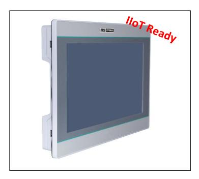
RS Pro IIoT HMI, types **215-6607** features remote monitoring, control & update from a PC via secure HTTPS protocol on a cloud server.
