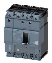
circuit breaker 3VA1 IEC frame 160 breaking capacity class H Icu=70kA @ 415V 4-pole, line protection TM220, ATFM, In=25A overload protection Ir=18A...25A short-circuit protection Ii=12.8 x In N conductor unprotected clamp connection
