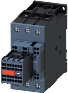
power contactor, AC-3e/AC-3, 51 A, 22 kW / 400 V, 3-pole, 20-33 V AC/DC, 50/60 Hz, with integrated varistor, auxiliary contacts: 2 NO + 2 NC, main circuit: screw terminal, control and auxiliary circuit: spring-loaded terminal, size: S2, captive auxiliary switch
