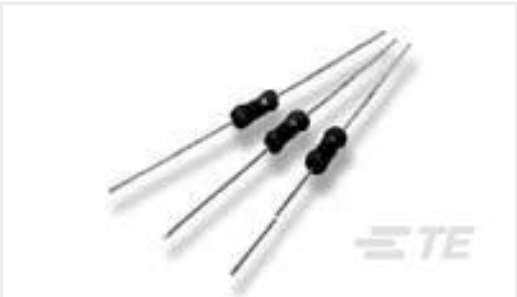
TE Part #2-1625892-8 3W SM M/OX 5% 20K
