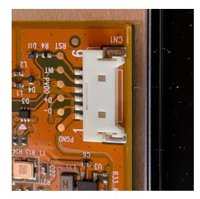
Note the correct orientation and then push the USB adapter cable connector into the display touch connector
