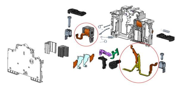
\*Rounded parts have soldered or riveted pieces that cannot be manually disassembled.
