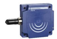
Inductive proximity sensors XS, inductive sensor XS7 80x80x26, PBT, Sn40mm, 12...24 VDC, M12
