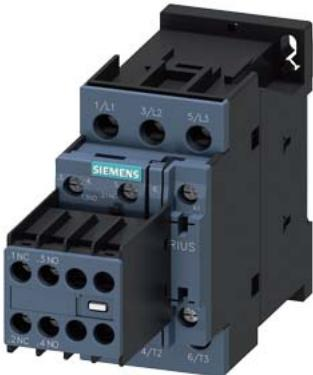
power contactor, AC-3e/AC-3, 17 A, 7.5 kW / 400 V, 3-pole, 42 V AC, 50 Hz, auxiliary contacts: 2 NO + 2 NC, screw terminal, size: S0, removable auxiliary switch
