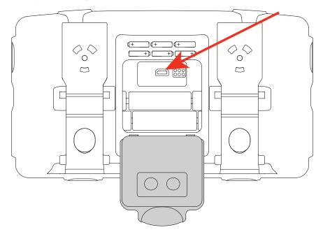
■ Simultaneously press the <sup>(1)</sup> button and the **MEM** key. The instrument displays **SOFt UPd**.
