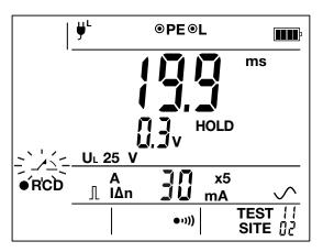
Press the TEST key again to return to voltage measurement.
