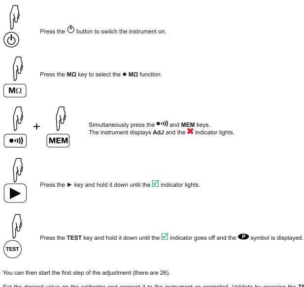
Set the desired value on the calibrator and connect it to the instrument as prompted. Validate by pressing the **TEST** key. The instrument displays **1** to indicate that it is performing the first step of the adjustment.
