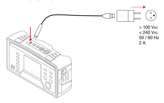
■ The instrument is switched on and the display unit indicates the progress of the charging.
