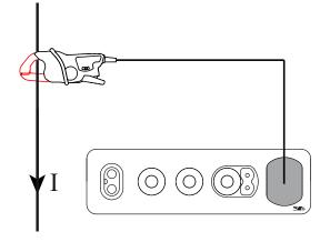
This current measurement can be made only in AC.
