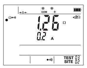
For as long as the measurement varies between some value and **OL**, the instrument remains on even if not in permanent mode.
