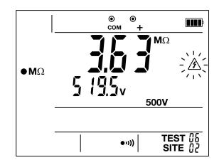
When you release the **TEST** button, the instrument displays **dIS** (discharge) to indicate that it is discharging the object tested. If the object is not capacitive, discharging is very rapid. When the voltage falls below 25V, the **dIS** and A symbols disappear from the display unit.
