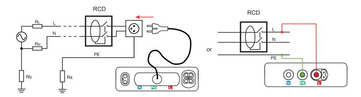
The instrument first of all checks that the voltage between the **L** and **PE** terminals is correct. If it is, the symbol lights steadily. If not, the symbol blinks and it is not possible to make a test. If  $U_{LPE} < 90$  V, the instrument displays  $U_{LPE}$  and  $U_{NPE in}$  alternation.
