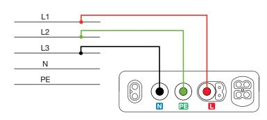
The phase-to-phase voltages are displayed, the values  $U_{12}$ ,  $U_{23}$  and  $U_{32}$  in cyclic succession, along with the direction of phase rotation,  $L_{3,L^2}^{L_1}$  or  $L_{1,L^2}^{L_3}$ .
