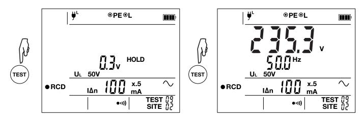
Press the **TEST** key again to return to voltage measurement.
