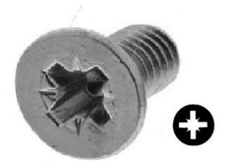
Countersunk, also known as Flat Head Machine Screws, are designed for ease of assembly and these machine screws with their cross recess drives are a popular driving method with this type of fastener as they allow the head to sink into the material. Machine screws can be used in pre-tapped holes or used with conforming nuts and washers in through holes.
