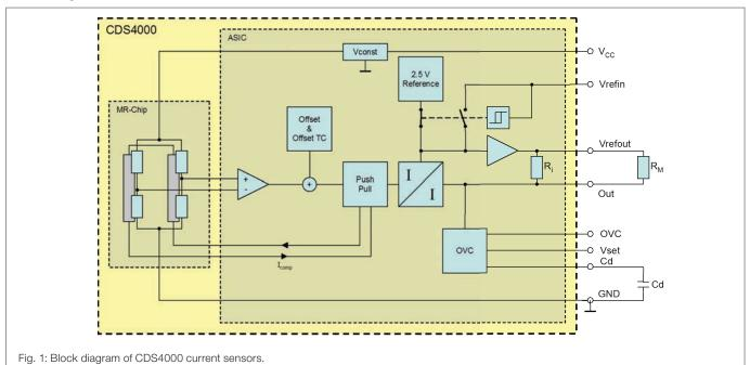
$<sup>^{2)}~~</sup>R_{_{M}} > 300~\Omega;$  reduces  $I_{_{PR}} but$  increases  $G_{_{V}}.$
