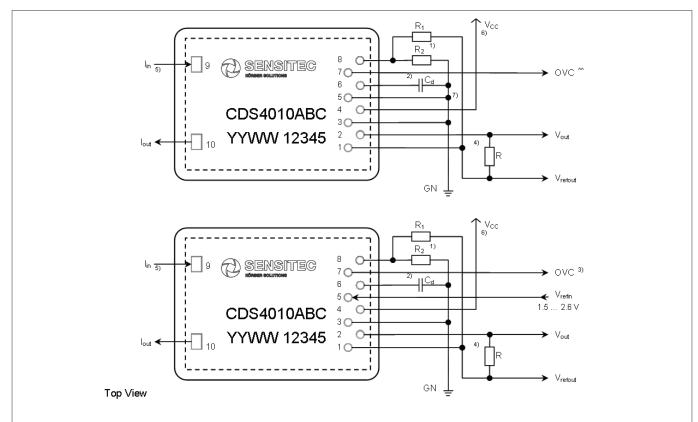
Fig. 7: *Top:* Example of how to use the internal reference voltage (pin 5,  $V_{refin}$  is routed on ground). *Bottom:* Circuit with external reference voltage at pin 5,  $V_{refin}$ .
