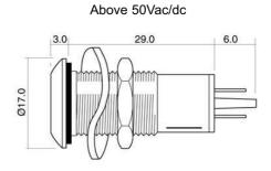
Dimensions in mm (Typical) Not to scale Anode termination indicated by red sleeve Mounting hole to be clean and burr free
