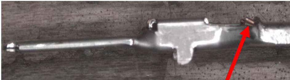
Excessive wire brush
